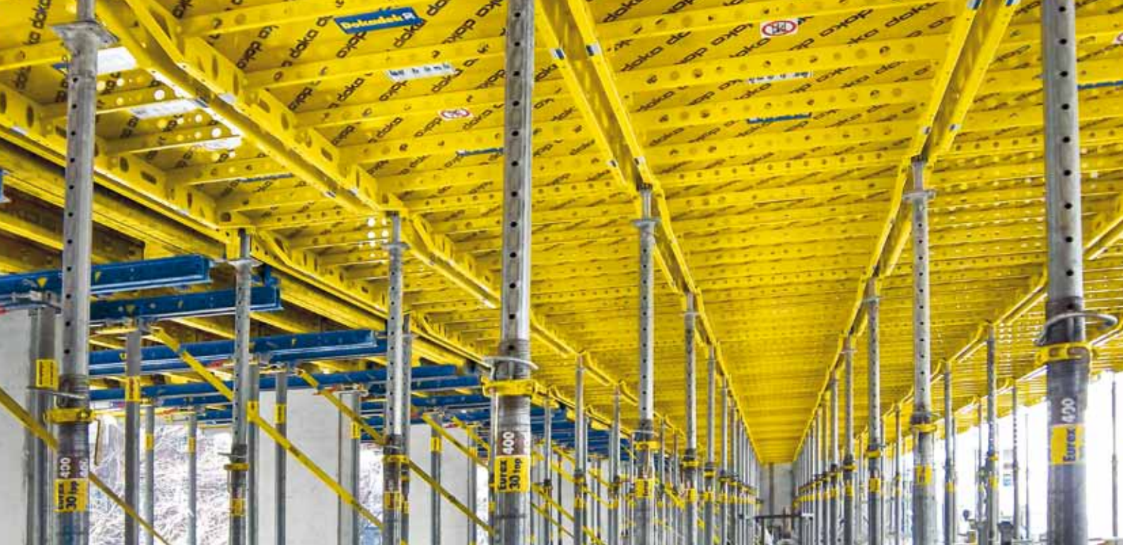
▲ The big, 3 m 2 Dokadek 30 panels make for high-speed forming of large areas, as there are far fewer parts to be shifted.
