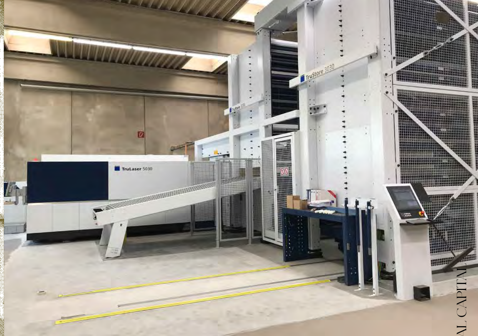
The new Trumpf fibre laser unit at umdasch The Store Makers in Leibnitz reduces the previous energy consumption of cutting work by half.
