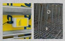
The cable sensor with lost cable has up to three measuring points and is positioned on the reinforcement before the concrete is poured.
