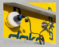
The accessories of the first version are compatible with the Concremote cable sensor 2.0.
