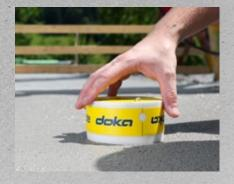
The Concremote slab sensor 2.0 is placed on the concrete immediately after the concreting work.
