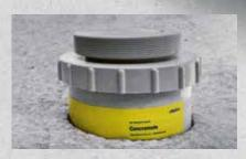
The slab sensor is placed on the surface of the fresh concrete after screeding.
