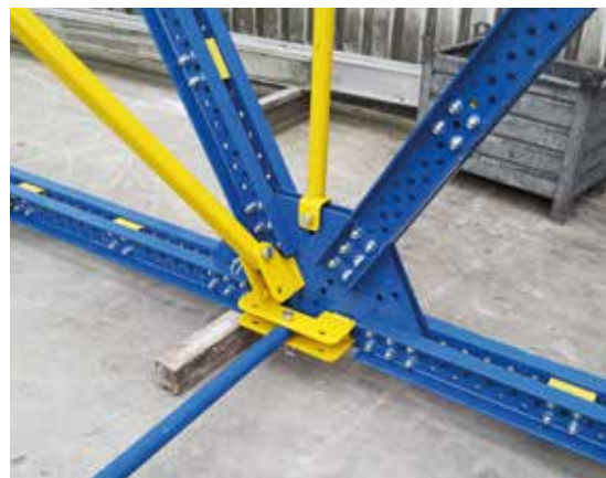
The three basic components of Doka UniKit: U-profiles, splice plates and struts
