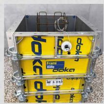
Calculation of concrete compressive strength in accordance with standards: EN 13670, DIN 1045-3, ZTV-ING, NEN 5970, NF EN 13670, BS EN 13670, BS 1881 part 201, ASTM C 1074 and ACI 228.1R
