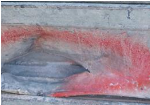
Length profile broken
