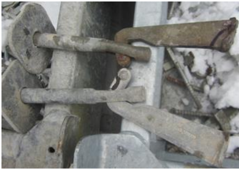
Connecting part bent
