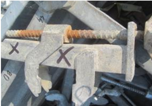
Connecting part bent
