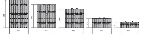
Optimum element size-grid with only two different widths of element (inside element 2.40 m, outside element 2.50 m)
