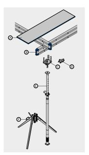
A Plywood B Doka beam H20 top16'- 0" and 11' - 6" C Lowering head H20 D Supporting head H20 DF E Doka floor props Eurex F Removable folding tripod
