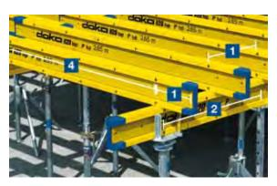
Marks on the beams allow for spacing props and stringers at a standard 4'  $\times$  8' grid with no measuring required
