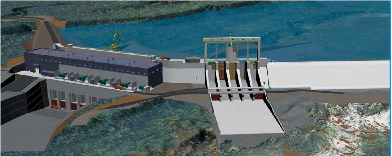
▲ View of Spillway Structure and Powerhouse - rendering by Nalcor Energy
