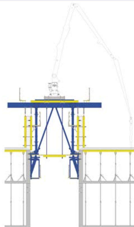
▲ A concrete placing boom can be integrated into the formwork and raised with the Doka Super Climber.
