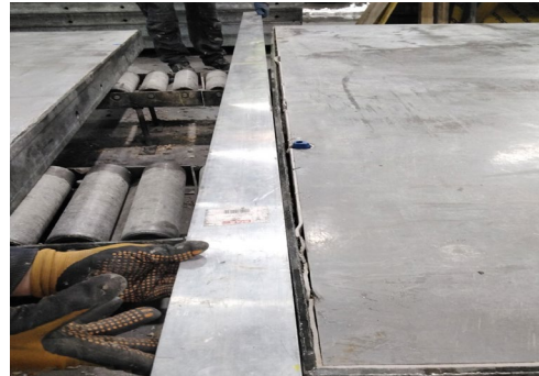
Length profile bent / panel deformation
