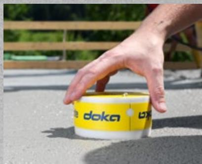
The Concremote slab sensor 2.0 is placed on the concrete immediately after the concreting work.
