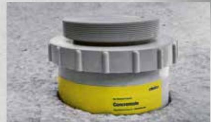
The slab sensor is placed on the surface of the fresh concrete after screeding.
