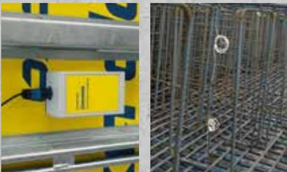
The cable sensor with lost cable has up to three measuring points and is positioned on the reinforcement before the concrete is poured.
