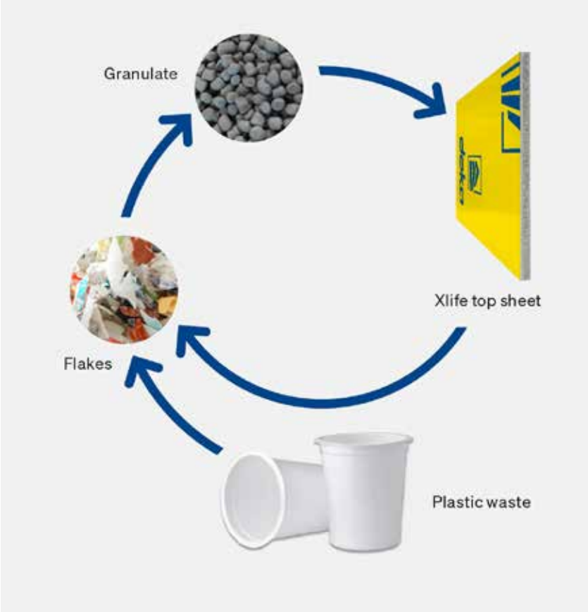
Produced from recycled plastic today – returned to the cycle at the end of its life. This is how formwork sheets gain multiple lifecycles.
